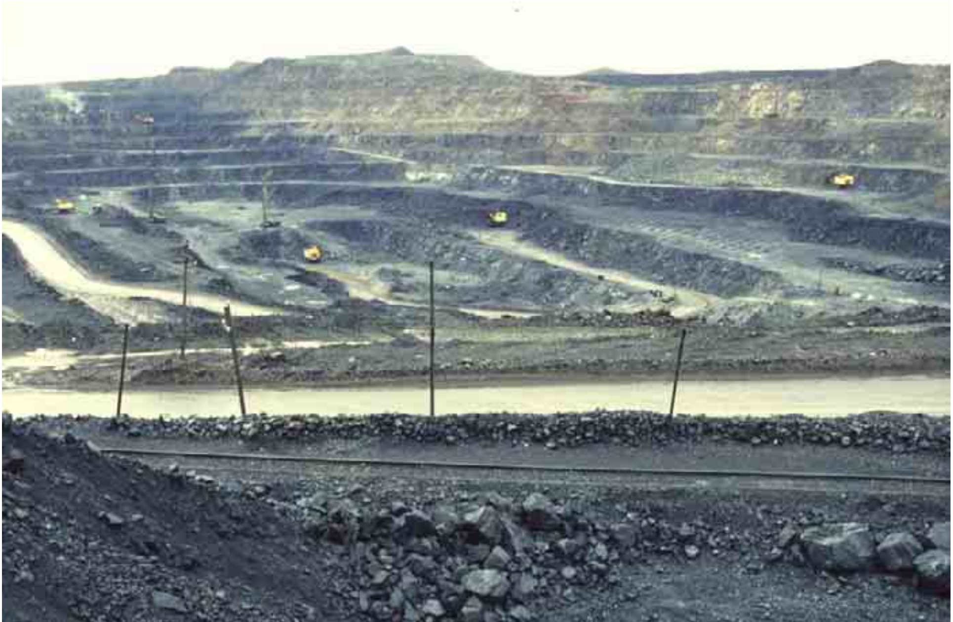
Bayan Obo, northern China: iron-REE ore open pit mining >60 Mt @ 35 % Fe, 4-5 % \text{Re}_2\text{O}_3
