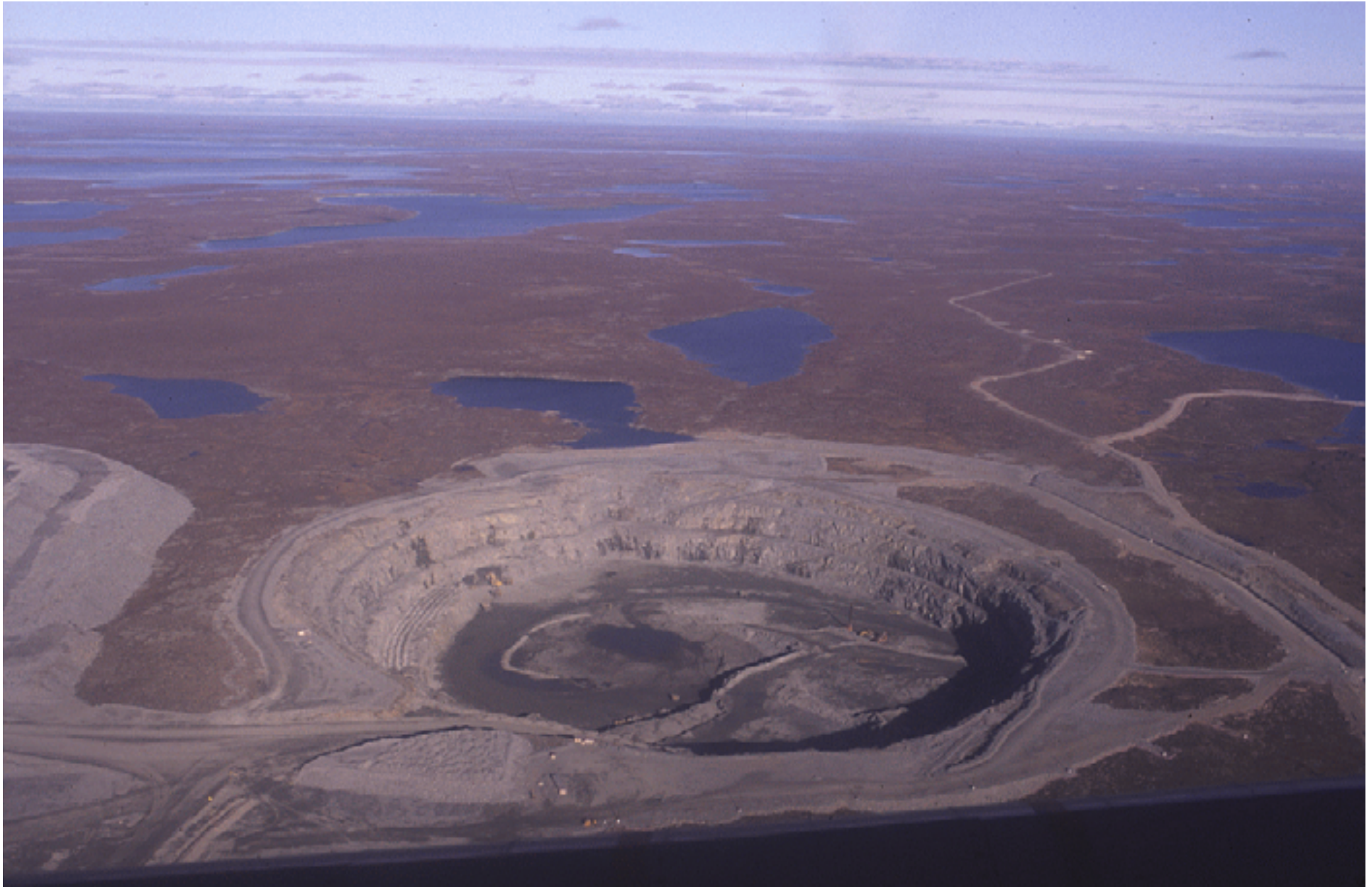
Ekati Mine (Sep 1999), 700 M USD, 3.6 ct/t @ 130 USD/ct Open pit mining from 1997 until 2003, now underground
