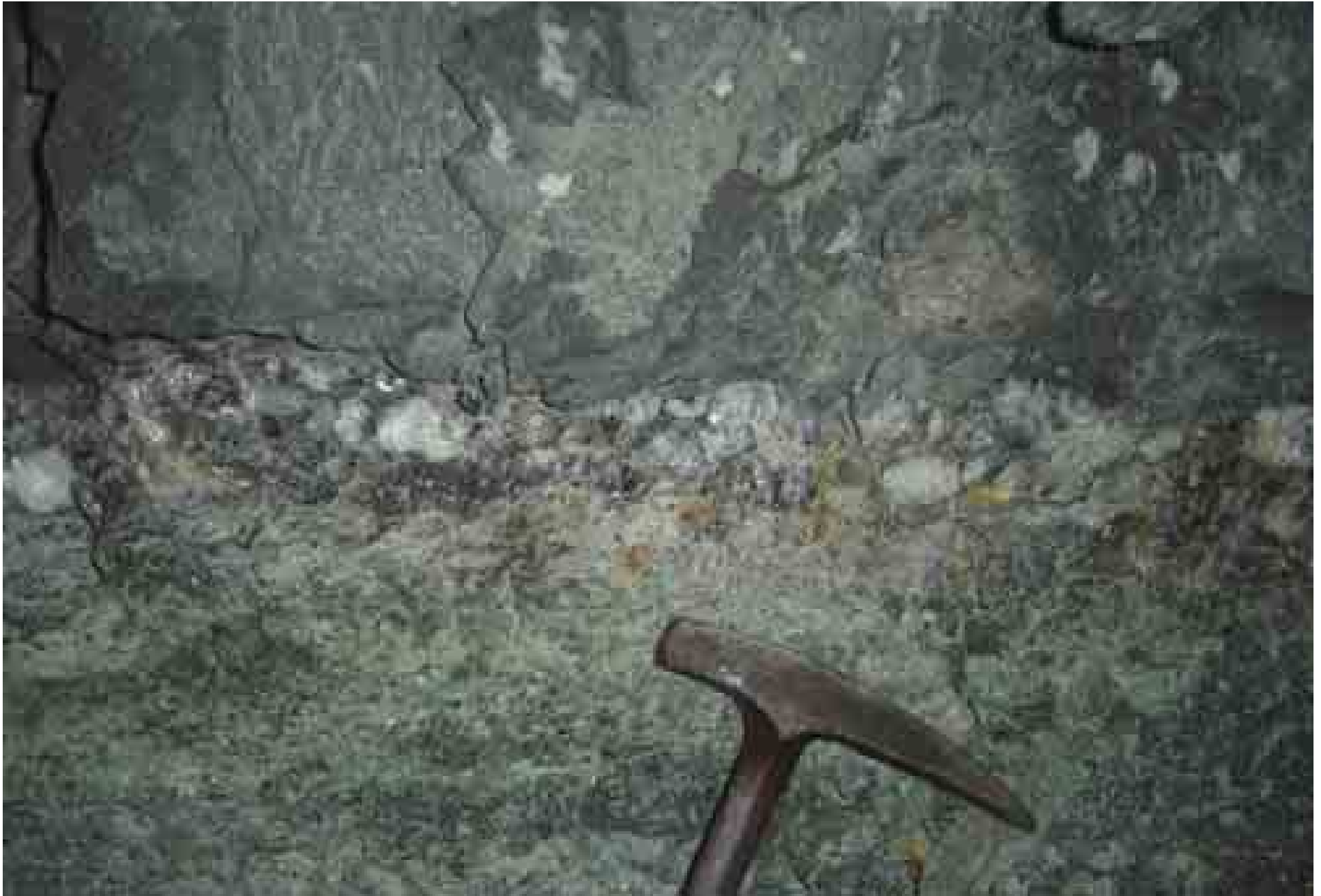
Mponeng mine: Ventersdorp Contact Reef (-3200 m), cut-off at 1000 g/t x cm Overlying meta-basalt: 2714 ±8 Ma (SHRIMP U-Pb on zircon)
