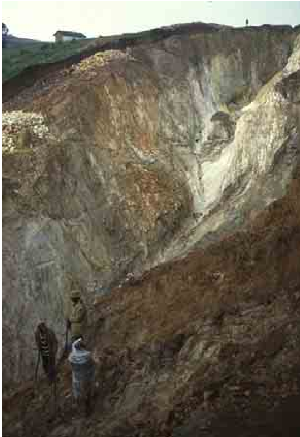
Kabarore rare-metal pegmatite, Burundi: ground sluicing
