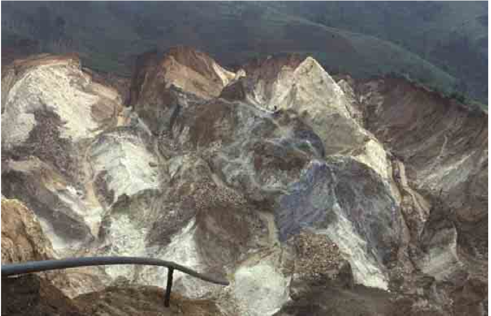
Kabarore rare-metal pegmatite, Burundi: ground sluicing
