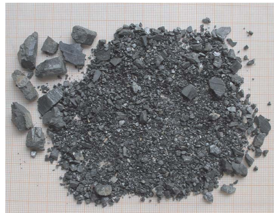
Fig. 2. Tantalum ore (called "coltan" in Central Africa) consists of the Ta-rich member of the columbite mineral group, (Mn,Fe)(Ta,Nb) 2 O 6 , which occurs as a black, heavy accessory mineral in rare-metal granite pegmatites.
