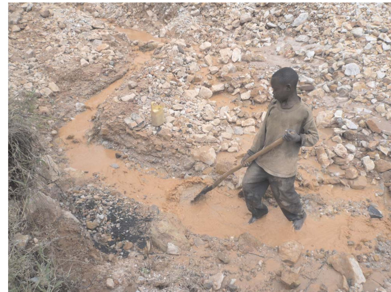
Fig. 4. Artisanal tantalum mining at smallest scale: Lonely young boy recovering a heavy-mineral concentrate by washing with a shovel in flowing water (Nkokwe, Gatumba district, Rwanda).
