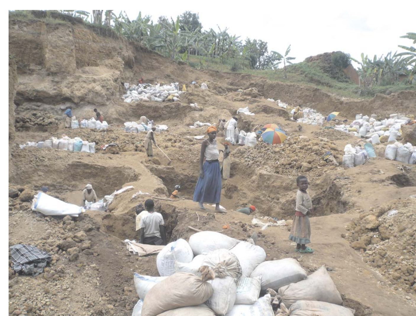
Fig. 9. Artisanal mining of Quaternary travertine terraces for liming of acid soils near Ruhengeri, northwestern Rwanda.
