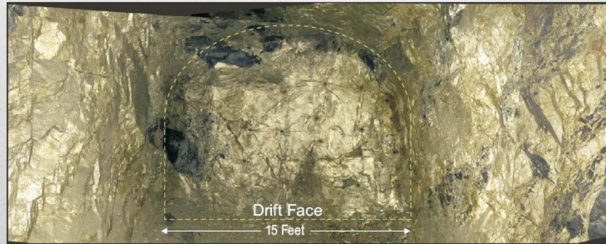
Podolsky Mine - 2450 Level drift intersecting massive Cu-Ni-Pt-Pd-Au mineralization with estimated grade of 20-25% Cu, 1-2% Ni, 0.25-0.75 opt TPM
