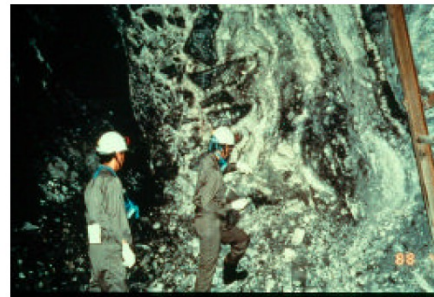
Photo 19. Banded adularia-sericite epithermal gold-silver fissure vein showing marginal floating clast breccias, Hishikari
